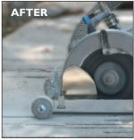
VACUUM REQUIREMENTS: SawVac™ will work with any vacuum, but for optimum efficiency use a vacuum rated at or above 11.5 amps (1.75 continuous hp) or 110 cfm.
