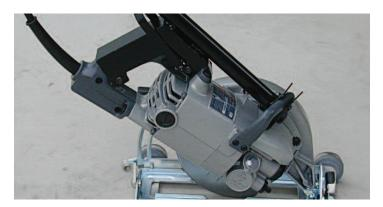
**USES:** ACCESS CUTS in slab concrete for retro plumbing and electrical; TENSION RELIEF LINES in slab concrete; SCORE DECORATIVE LINES in poured slab or overlays.
