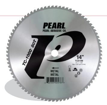
Pearl's Titanium Carbide Tip Metal blade (TC-1000<sup>™</sup>) is designed to cut a variety of mild ferrous metals with fewer burs, less dust and reduced material burning than abrasive products. It provides much longer life than traditional abrasive wheels. The Pearl TC-1000<sup>™</sup> is engineered with a triple chip design for added
