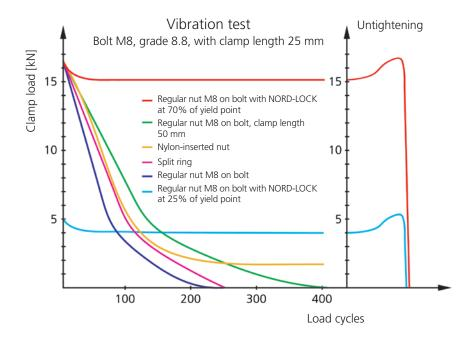
The diagram displays NORD-LOCK's superior performance. Most of the commonly used locking devices show limited or no holding performance when exposed to vibration. Whereas bolted joints secured with NORD-LOCK washers only lose some of the initial preload due to normal settlements between the contact surfaces. NORD-LOCK's unique wedge-locking function is proved by the clear increase in clamp load during untightening.
