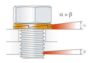
When the bolt and/or nut is tightened the teeth of the NORD-LOCK washers grip and lock the mating surfaces allowing movement only across the cam faces. Any rotation of the bolt/nut is blocked by the wedge effect of the cams. NORD-LOCK safely secures bolted joints exposed to vibration and dynamic loads.
